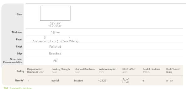
Product and Installation Details | ANSI A108.02 Section 4.3.8.2 - For running bond/brick joing patterns utilizing tiles (square or rectangular) where the side being offset is greater than 18" (nominal dimension), the running bond offset will be a maximum of 33% unless otherwise specified by the tile manufacturer. If an offset greater than 33% is specified, specifier and owner must approve mock-up and lippage.
