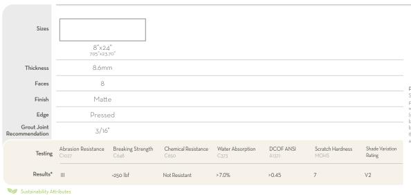
Product and Installation Details | ANSI A108.02 Section 4.3.8.2 - For running bond/brick joing patterns utilizing tiles (square or rectangular) where the side being offset is greater than 18" (nominal dimension), the running bond offset will be a maximum of 35% unless otherwise specified by the tile manufacturer. If an offset greater than 33% is specified, specifier and owner must approve mock-up and lippage.
